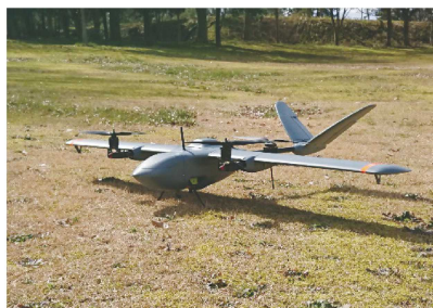
Fig.2 Fixed wing/vertical takeoff drone FUTVTOL-1
