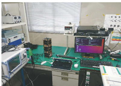
Fig.1 Functional test of micro satellite FUT-SAT-1
