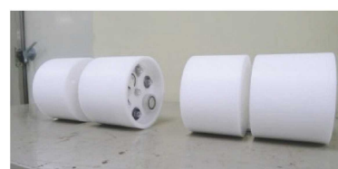
Fig.3 Photonuclear reaction X-ray spectrometer The amount of photonuclear reaction neutrons in each spectral bin is measured with a bubble neutron detector.
